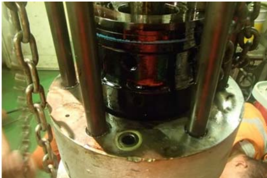
写真-4 HousingからBarrelを抜き出し中 Photo-4 Barrel Being Removed from Housing
